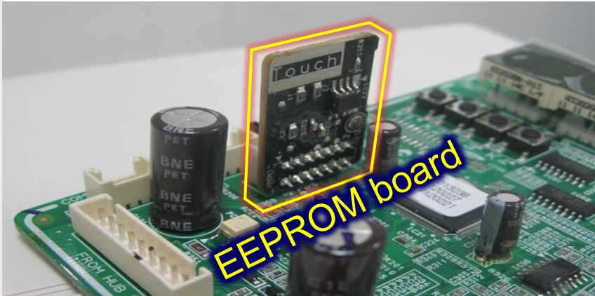
Outdoor unit main PCB
