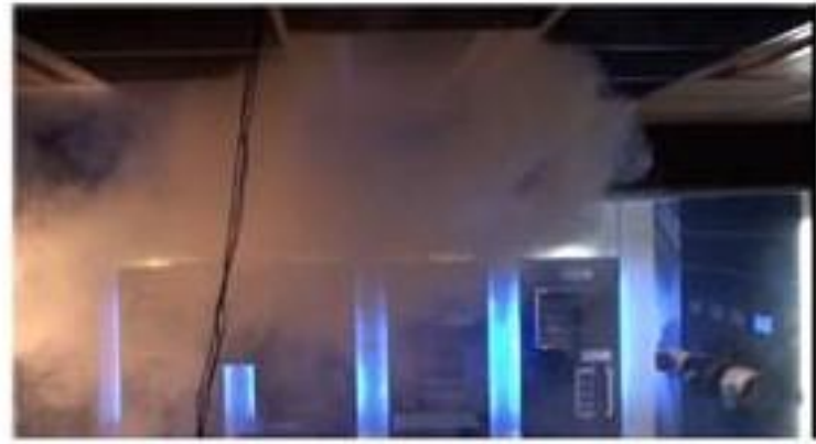
Figure 2: Without Varyset; V = 15 \text{ l/s} ; \Delta t = -12 \text{ K} Dumping is evident.
