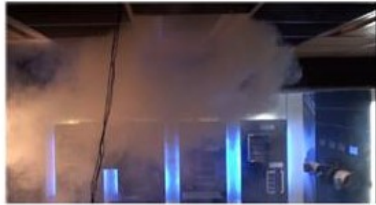
Figure 2: Without Varyset; V= 15 l/s; \Delta t= - 12 K Dumping is evident.
