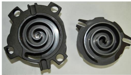
Top fixed scroll Bottom orbiting scroll
