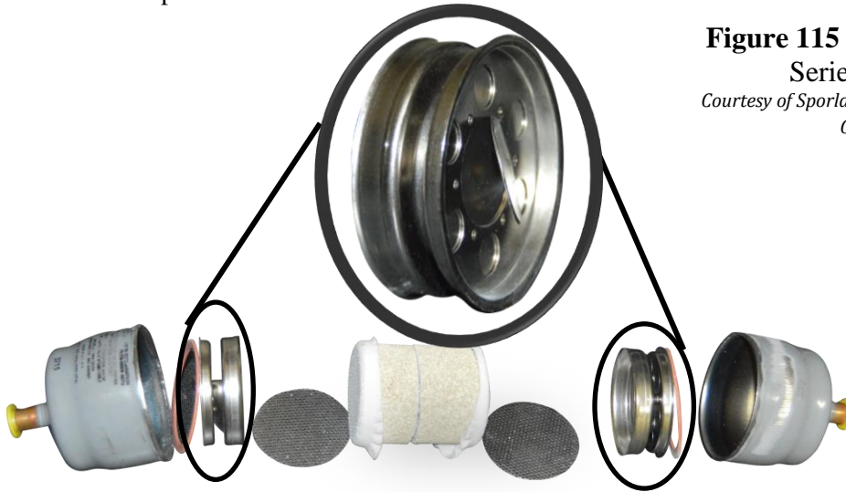
Figure 116 - Filter Drier Bi-Directional Internals
