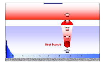
Chilled Beam Displacement ventilation creates a single vertical passage of fresh air through the breathing level, eliminating horizontal cross transmission of respiratory pollutants and associated contagious disease.
